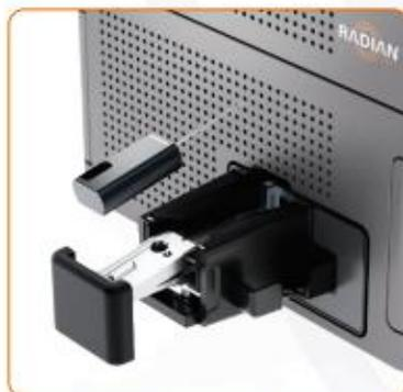
3. Insert capillary to start acquisition
